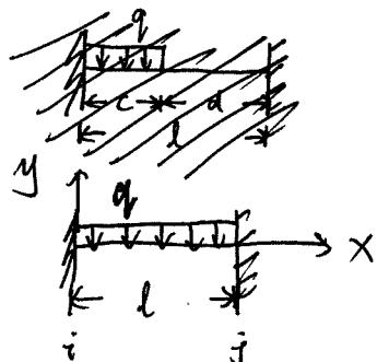
$$\text{局部坐标系下单元的固端内力 } \{F'_0\}^{\circledR} = \begin{pmatrix} \{F'_{0i}\}^{\circledR} \\ \vdots \\ \{F'_{0j}\}^{\circledR} \end{pmatrix}$$
